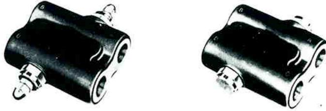
The CROSS series RC differential - poppet type double relief valve has been designed to protect equal displacement cylinders or motors from external or shock loads. Fluid which passes through one relief valve flows directly to the opposite side or circuit of the valve, thus preventing cavitation of the cylinder or motor as a result of relief discharge. These units incorporate the same hydraulically dampened poppet design as the RD series units.
